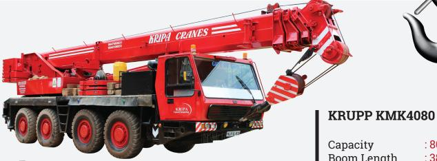
Capacity :80 MT Boom Length : 38 Mtrs Fly Jib Length : 16 Mtrs
